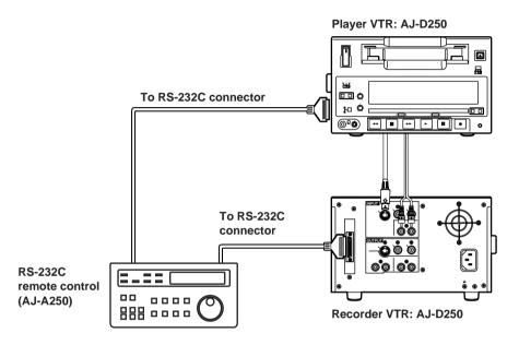
• Set the INPUT SELECT switch to the position which corresponds to the connection with the player VTR.
